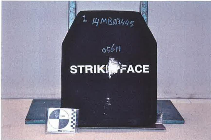
Figure 1 : Strike face, Sample 14MB03445 after the test.
