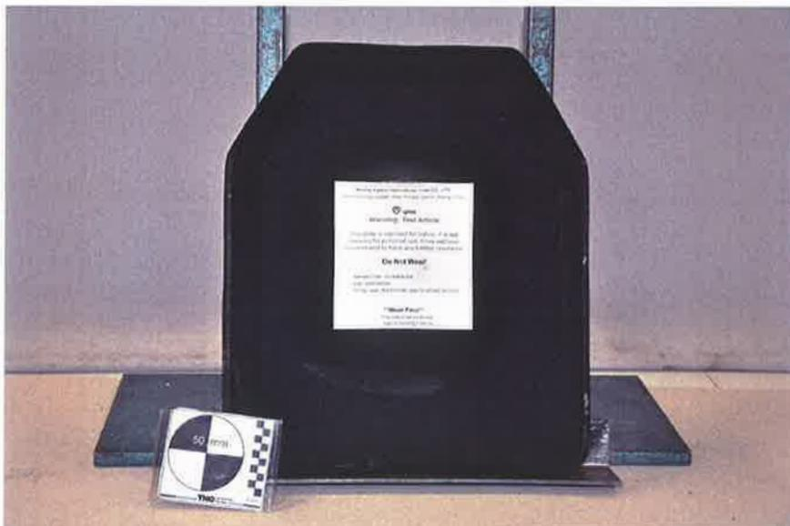
Figure 2 : Body Side, Sample 14MB03445 after the test.
