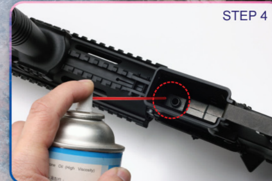
Use Airsoft Safe Silicone to lubricate the hop up chamber. Use silicone lubricant sparingly..
