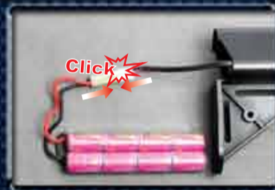
Connect battery plug with the connector until you heard a click sound.
